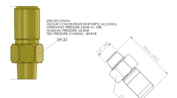
Odouriser NF361076 and specification (top left), odouriser in position it should be fixed in (bottom right)
